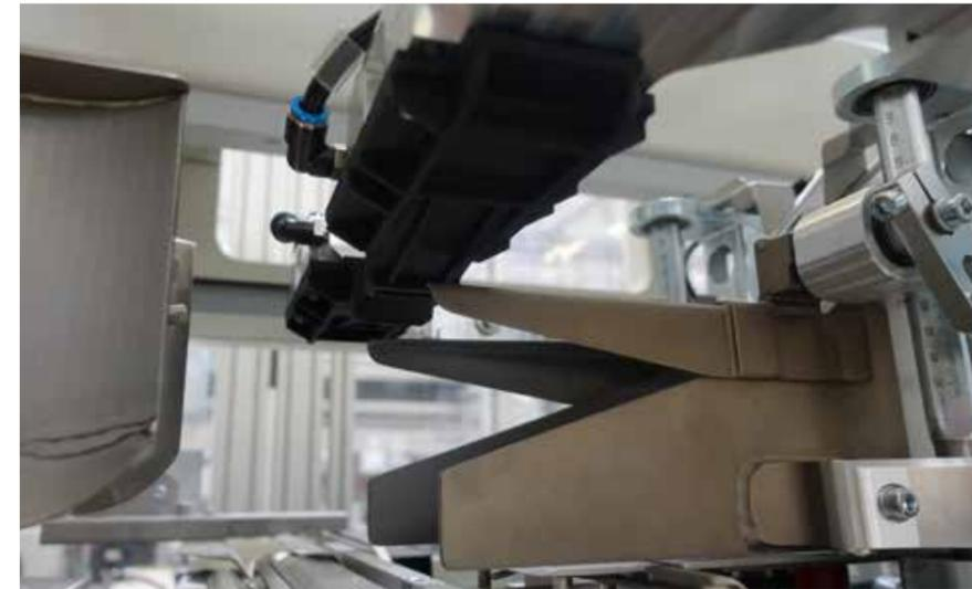
◀ The bag suction in the bag intake module was manufactured by 3D printer. With this process, parts can be produced quickly and flexibly. In addition, 3D printing technology has been used to optimize the airflow of the interior.
