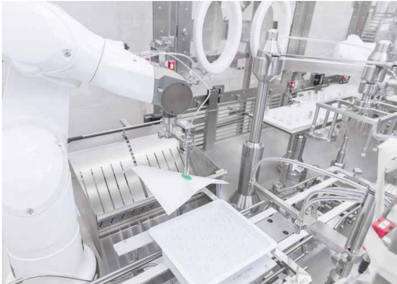
Robots manage fine movements, for example removing the Tyvek foil that protects sterile containers.
