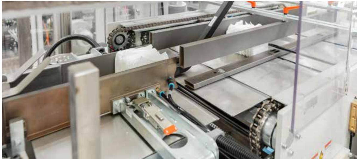
▶ The special edition Pearl contains many frequently requested functions as standard. Here is the main compression of the products, which can easily be exchanged for a rotating cassette. For example, the shortened web conveyor on the right saves costs and reduces the overall length of the system.
