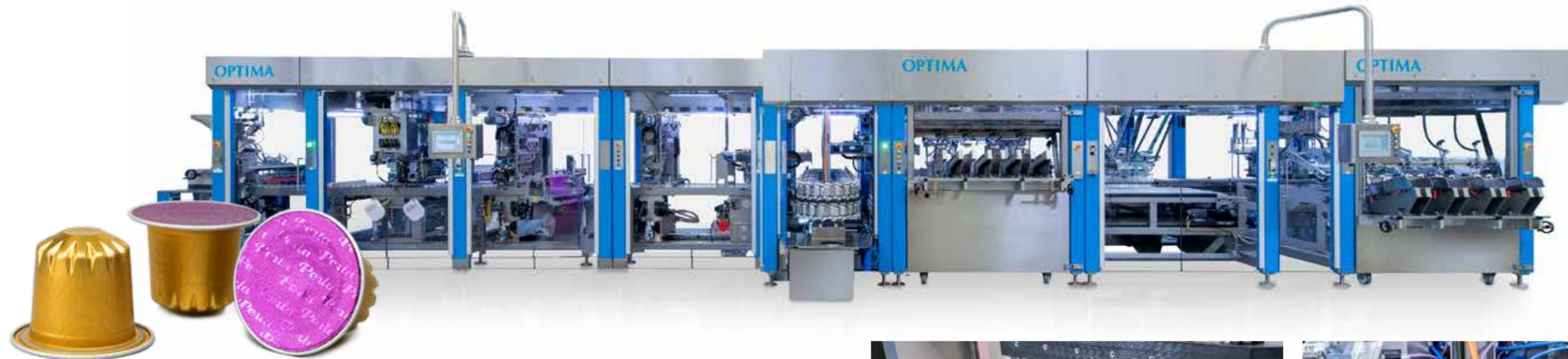
← Together, the OPTIMA CFL (left) and the OPTIMA CBF (right) make a powerful combo for filling and packaging coffee capsules.
