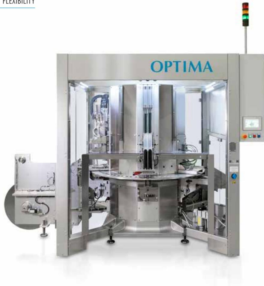
Focus on process safety: When the capsules are stacked, an optical presence check ensures that all transport plates are loaded.
