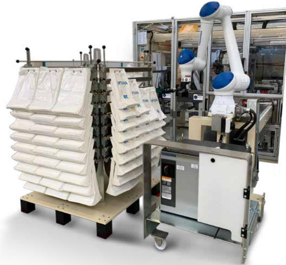
The trend towards fully automated systems is creating new areas of use for robots, such as placing stacks of bags on the bag conveyor. Optima Nonwovens' extremely efficient solution requires no additional security systems like scanners or safety sensors.
