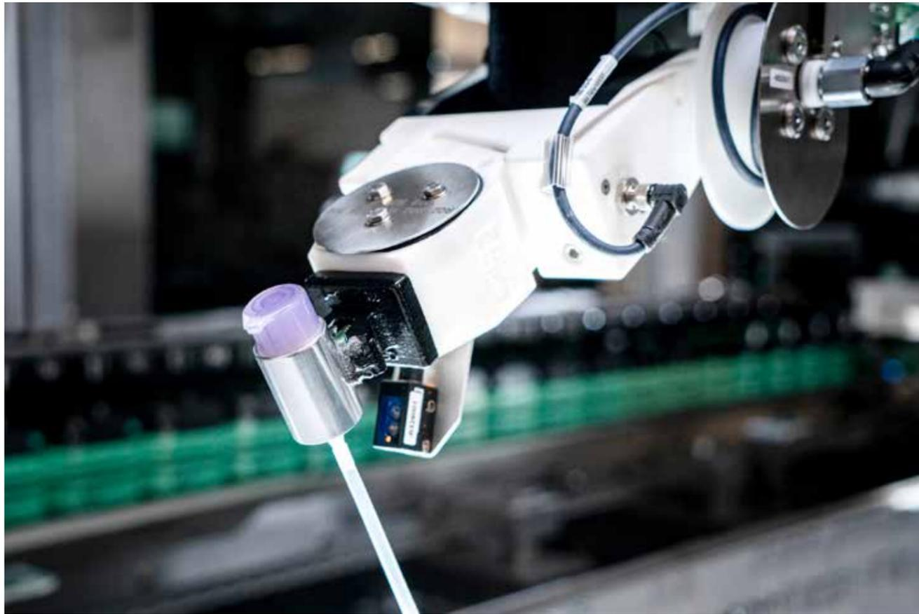
Optima uses 3D printing to rapidly adapt robotic systems to new formats. If required, new format sets can be printed out at the location where they will be used.
