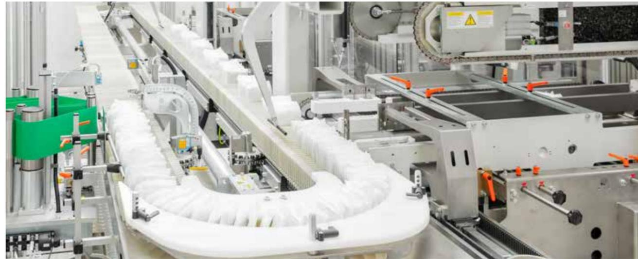
◀ The dual-discharge system means that twice the output can be achieved with more stable packaging processes. For single-row packs, the product formation is transferred without stopping by the Robot Pusher on the web conveyor.
