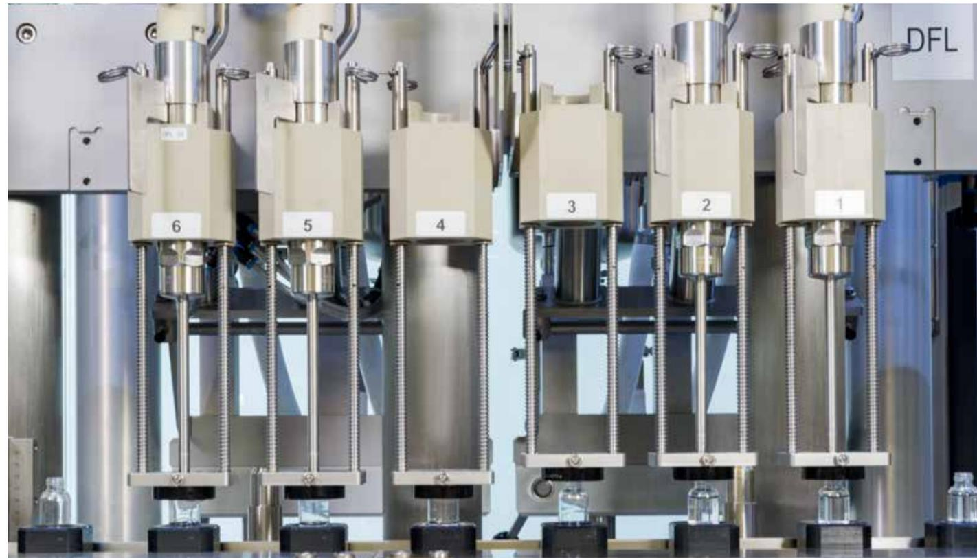
➤ A filling system that can handle both single- and two-phase products.
