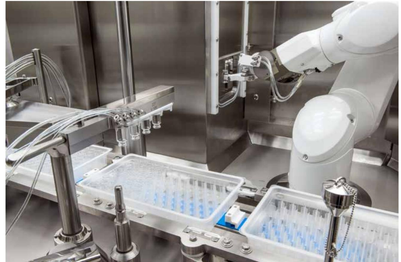
The OPTIMA MultiUse Filler combines numerous robotic systems. These include a de-nesting robot that supplies various containers to the filling and closing process.
