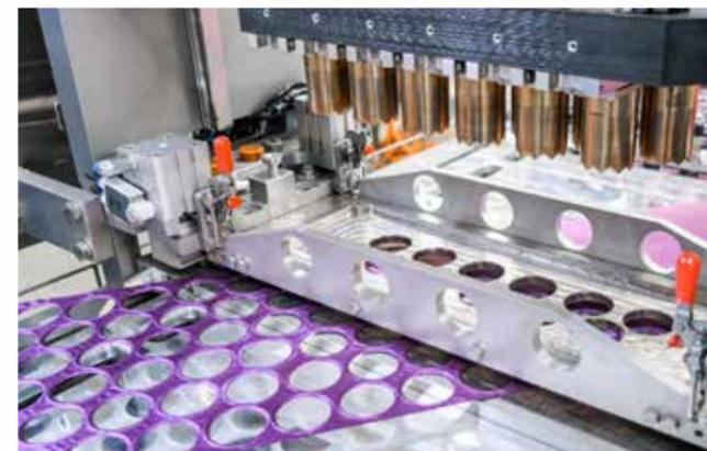
^ Optimum material utilization is assured because the film for sealing the capsules is fed in at an angle and with a punched offset.
