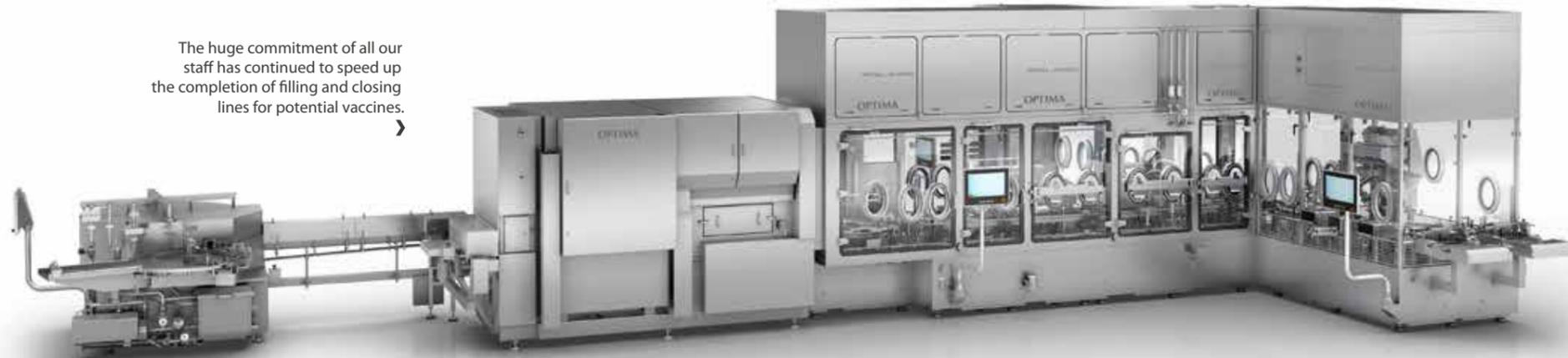
During the crisis, machine solutions like the OPTIMA ImmuFill® were in particularly high demand. This solution enables the filling of reagents for diagnostic test kits.
