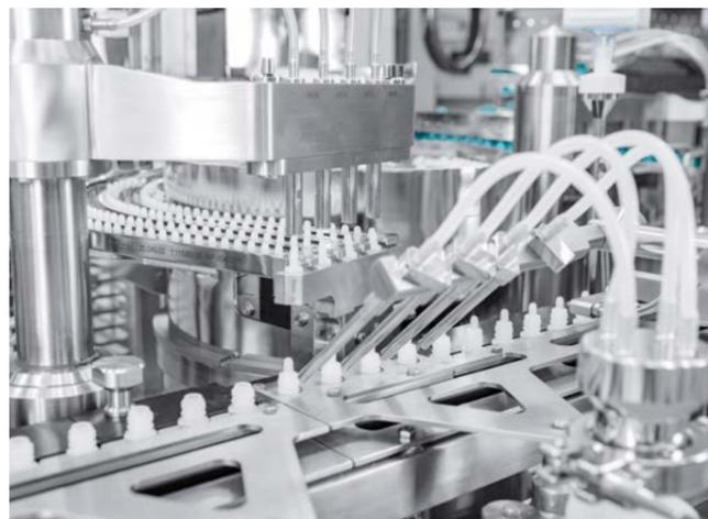
› Four headed filling systems: Concealed on the left are the stacked peristaltic pumps. Also installed – rotary piston pumps to process viscous products.
