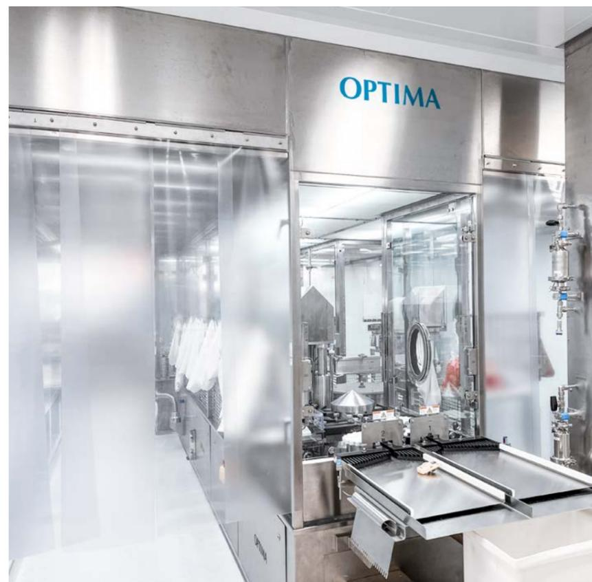
^ The line is operated with an Active Open RABS and under numerous laminar flow units in cleanroom class B.
