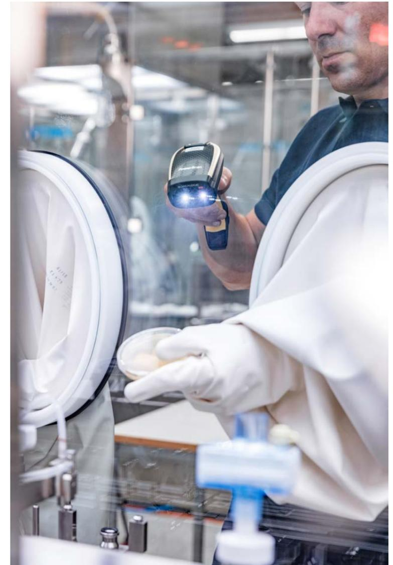
Using a new digital solution from Optima Pharma, agar plates can be scanned and unequivocally assigned. In addition, timing functions are also integrated.
