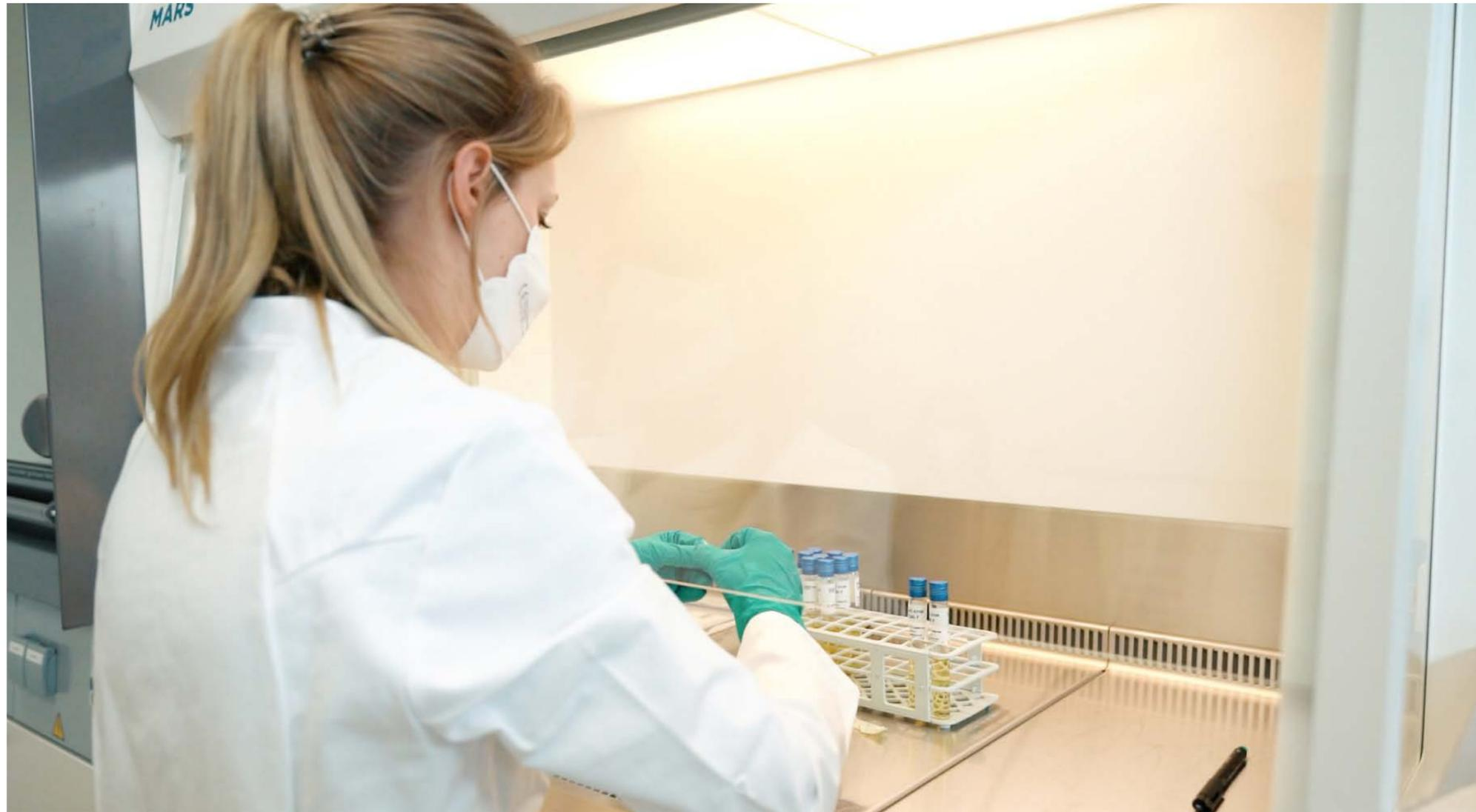
In the CSPE Center laboratory at Optima: Biological indicators in a nutrient solution with a positive and negative specimen are prepared for incubation during cycle development. The complementary application of enzyme indicators for this process is rational. Metall+Plastic in cooperation with Protak Scientific researched application potentials.
