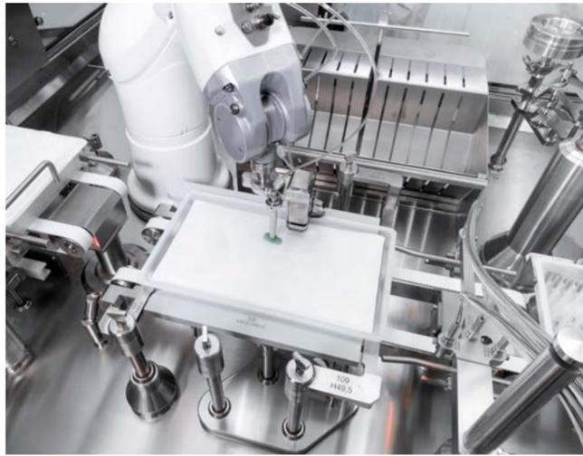
^ Nested containers are unpacked automatically. Bulk containers such as non-pre-sterilized vials can optionally be fed via a second product path.
