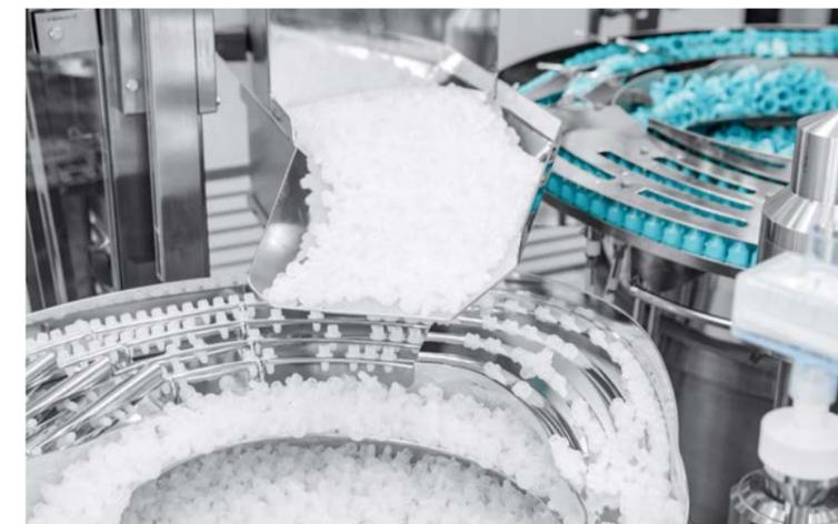
◀ The sorting devices ensure the correct alignment and feeding of closures. The preservative free OSD technology is easily processed with dedicated change parts
