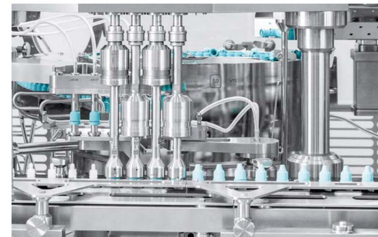
◀ A two-headed closing station ensures the caps are applied correctly, with the correct amount of torque for easy opening.
