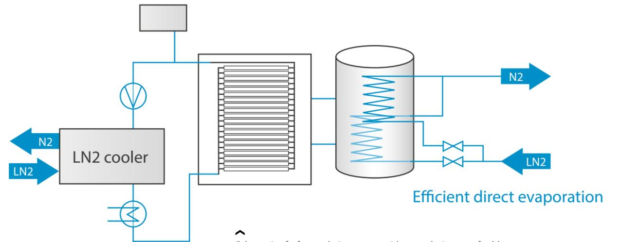
^ Schematic of a freeze-drying system with an explosion-proof cold cascade system. Both components – freeze-drying chamber with shelves and ice condenser – receive cold air from a central cooling system via heat exchangers and fluids in their own circuits.
