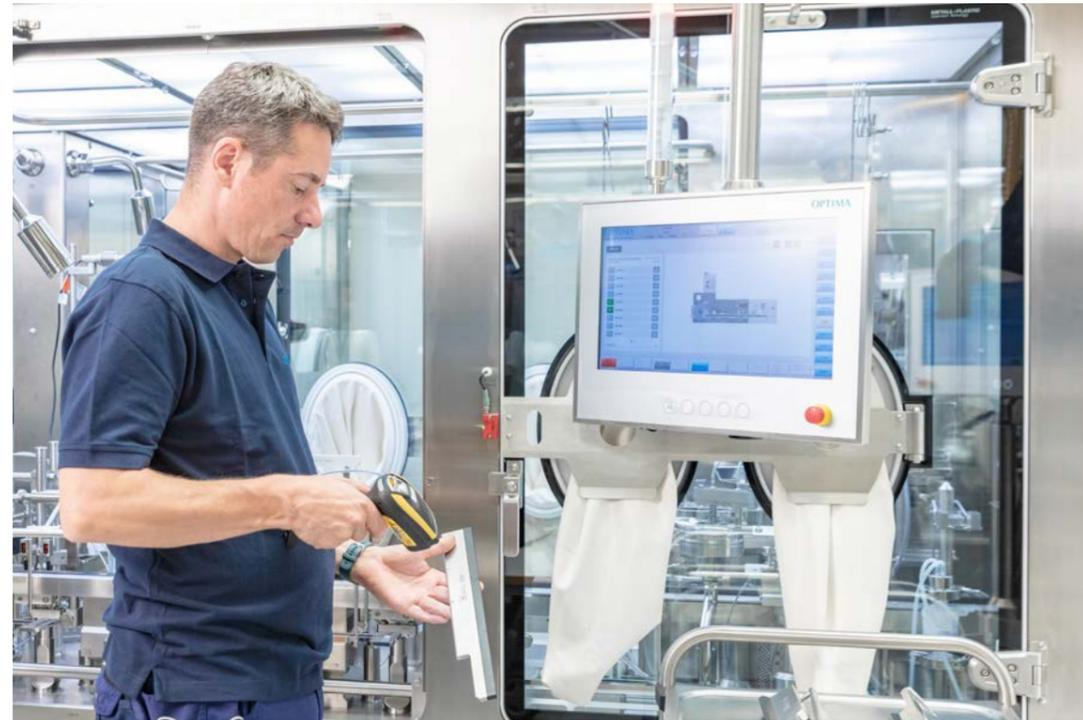
Production stops due to operating errors are costly in the pharmaceutical industry. A remedy is a digital format change assistant from Optima Pharma. As an option, format parts to be changed can be scanned, which increases process security.
