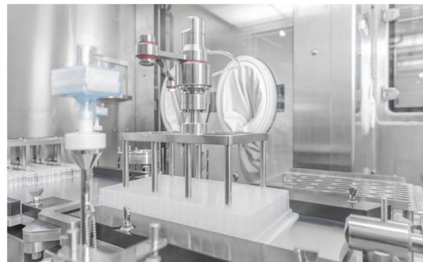
Vial trays are automatically removed with a robot before being moved into a linear infeed system.
